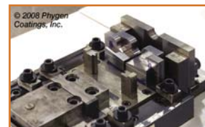
Glacier recently began assigning part numbers to elements of its quick change tooling. The shinier sections to the right are polished and coated with Phygen's FortiPhy™ CrN coating.
