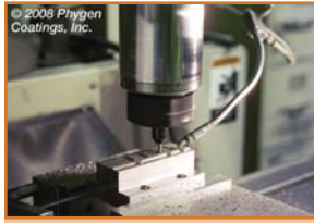
In the Glacier Caldwell tool room a groover die is being machined on this computer-controlled vertical milling machine.
